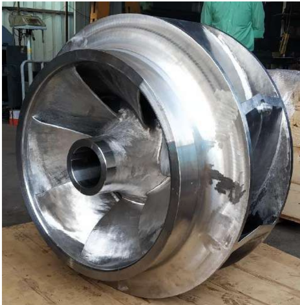
36/36 DV Lonovane - Cooling Tower Impeller, CFCL-Kota
