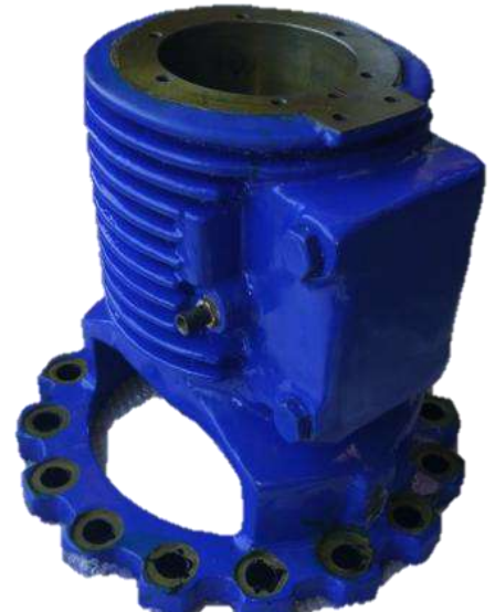
Modified Bearing Housing to reduce Bearing Temp CFCL
