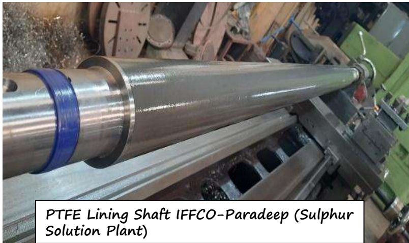
Single Piece ∅ 280x4m long Shaft
