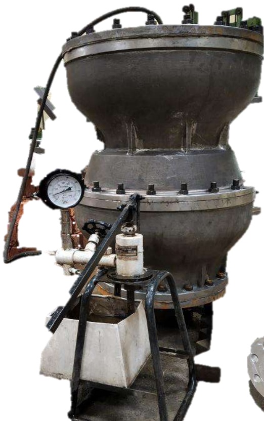
Bowl Assy Pressure Test, For Nayara Energy
